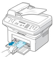
If there is any resistance and the paper does not move when you pull, or if you cannot see the paper in this area, check the fuser area around the toner cartridge. See page 9.3.
